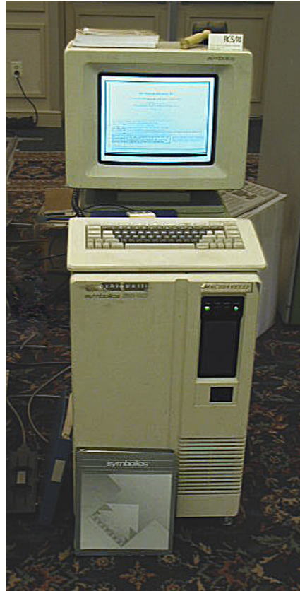
Figure 1.3: A Symbolics Lisp Machine, a specialized hardware platform designed to run expert systems which are a version of AI focusing on answering questions to challenging problems. a
